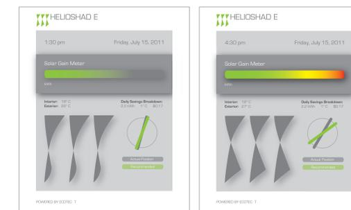
A simple display screen alerts the user when solar gain is reaching high levels. The colour threshold display changes from green to yellow to red as it calculates the amount of harmful light based on the time of day, season, geographic location and room size. This data calculation could potentially be powered by the Autodesk Ecotect program.
